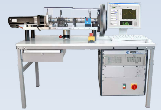
Torque Calibration System for Bottom Bracket Bearings
