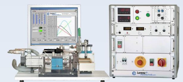
Motor Test Bench
